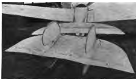
VIEW OF THE 1910 NIEUPORT MONOPLANE FROM BEHIND, SHOWING THE TAIL, FISH-LIKE BODY, AND WINGS
